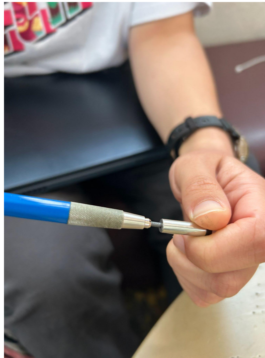
Figure 8: This user (Interviewee 7) has a mechanical pencil which has thicker lead that can be sharpened from a sharpening tool attached to the back of the pencil.
