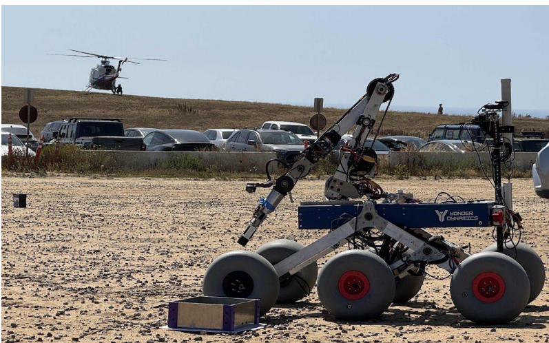
COMPETITION ROVER, URC · HARMONIC DRIVE JOINT
